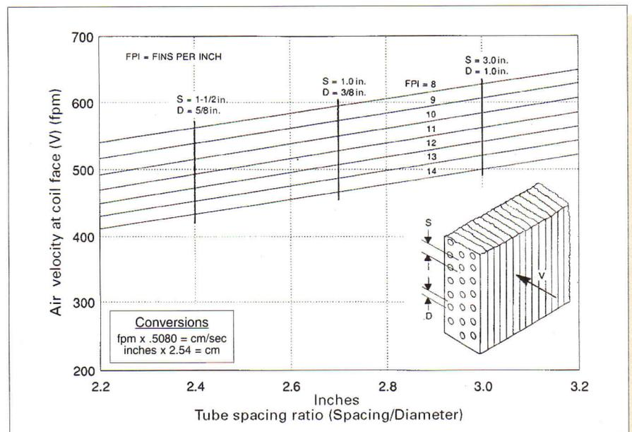
**FIGURE 1:** Coil face velocity above which condensate carryover occurs; typical cooling coil.
