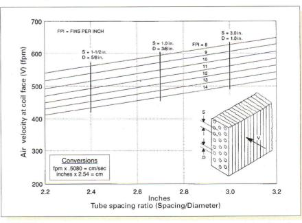
FIGURE 1: Coil face velocity above which condensate carryover occurs; typical cooling coil.
